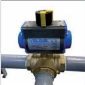
**PNEUMATICALLY OPERATED 3-WAY VALVES**
